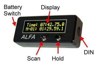
and selecting various options. Refer to the illustration for the location of all controls, connections and displays:
